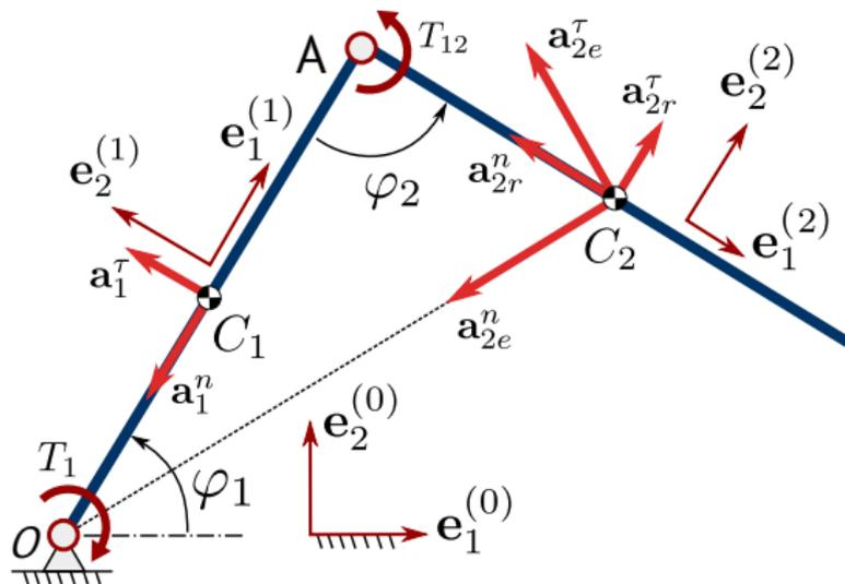
$$\mathbf{a}_2 = (\mathbf{e}_2^{(1)} 2L_1 + \mathbf{e}_2^{(2)} L_2) \ddot{\varphi}_1 + (-\mathbf{e}_1^{(1)} 2L_1 - \mathbf{e}_1^{(2)} L_2) \dot{\varphi}_1^2 + \\ + \mathbf{e}_2^{(2)} L_2 \ddot{\varphi}_2 - \mathbf{e}_1^{(2)} L_2 \dot{\varphi}_2^2 - 2\mathbf{e}_1^{(2)} \dot{\varphi}_1 L_2 \dot{\varphi}_2 = \begin{bmatrix} \mathbf{s}_{21} & \mathbf{s}_{22} \end{bmatrix} \begin{bmatrix} \ddot{\varphi}_1 \\ \ddot{\varphi}_2 \end{bmatrix} + \mathbf{f}_2$$
