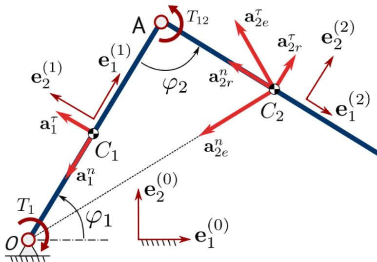
$$\mathbf{a}_1 = \mathbf{a}_1^n + \mathbf{a}_1^r = \mathbf{e}_2^{(1)} L_1 \ddot{\varphi}_1 - \mathbf{e}_1^{(1)} L_1 \dot{\varphi}_1^2 = \begin{bmatrix} \mathbf{s}_{11} & \mathbf{0} \end{bmatrix} \begin{bmatrix} \ddot{\varphi}_1 \\ \dot{\varphi}_1^2 \end{bmatrix} + \mathbf{f}_1$$
